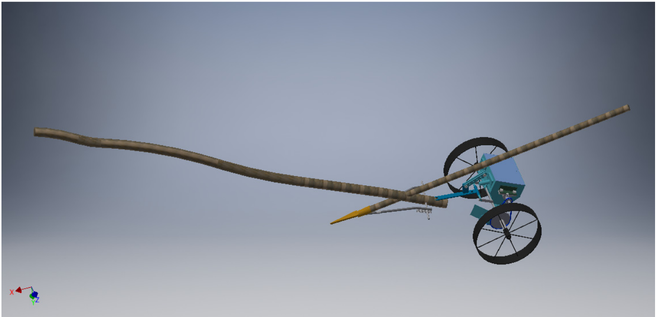
Figure 1. Isometric drawing of the designed tillage-cum-planter
