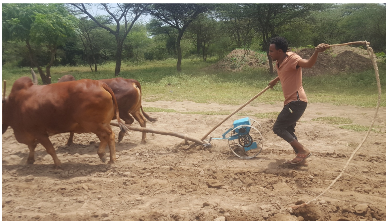
Figure 4. the developed tillage-cum-planter in operation
