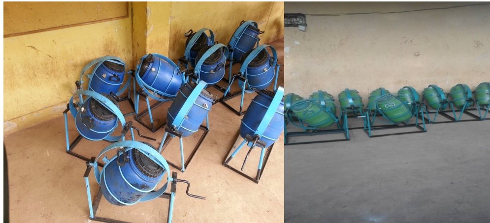
a. Capacity 20liters (Tocha) b. Capacity 15liters (Konta) Figure 1 , a and b. Improved milk churners
