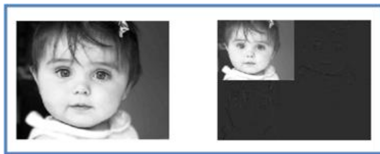
(a) (b) Figure 1. (a) Original image of baby, (b) result after the one-level 2-D Haar-DWT
