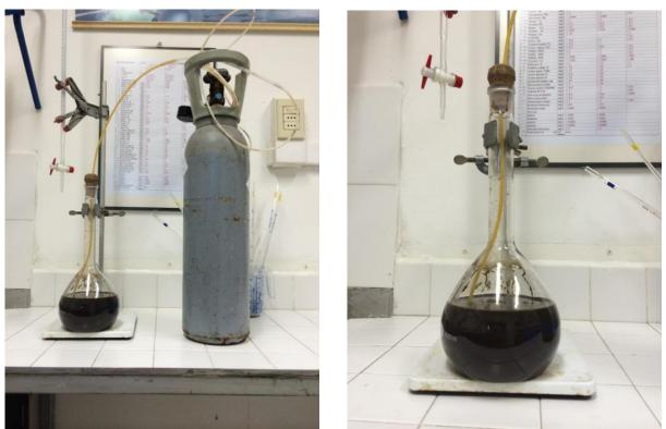
Figure 1. Lab set-up for the study of CO<sub>2</sub> chemical sequestration in piggery wastewaters.
