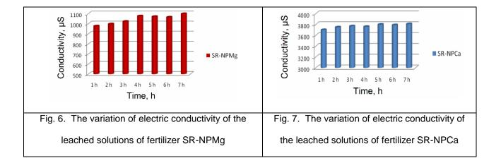
N-P-Ca is very small and is around 3700  $\mu$ S / cm for the extract obtained after 1 h and 3800  $\mu$ S / cm for the one obtained after 7 hours of extraction. The values at times 5, 6 and 7 had minor variations, only 10  $\mu$ S / cm (Figure 7).
